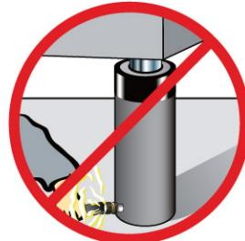
Never attempt to disconnect hydraulic hoses, fittings or couplers under pressure. Unload the ram, open the release screw on the hand pump and shift or open all hydraulic controls several times. If system includes a gauge, double check the gauge to insure pressure has been completely released.
