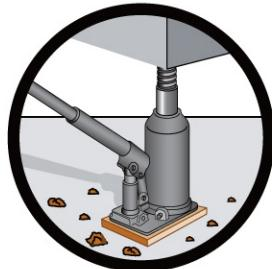
Every jack or ram, whether used individually or in a system, should be completely supported on a solid, firm, non-sliding foundation capable of supporting the load.
