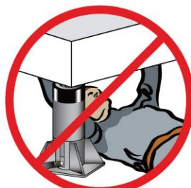
Hydraulic rams are not meant to be used as permanent supports, but are designed to lift and lower. If you need to hold the load for any length of time, cribbing or Simplex locknut cylinders should be used.
